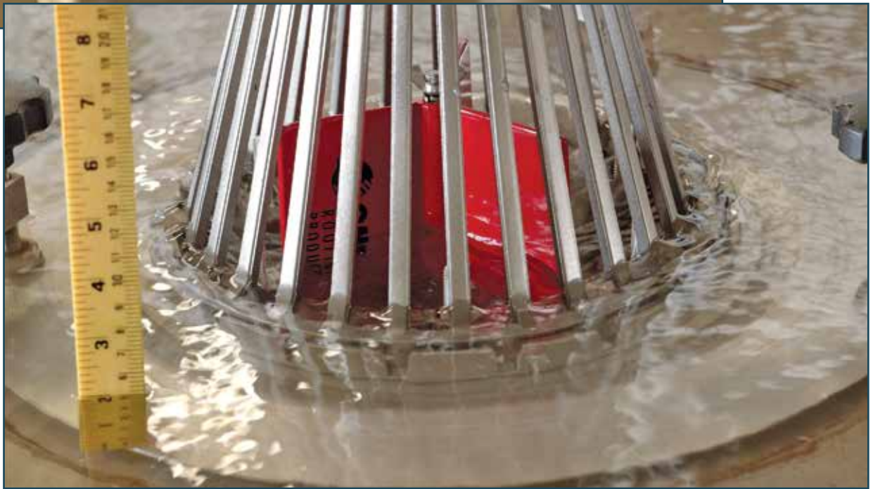
Figure 6 – A patented roof drain featuring a vortex breaker within a drain flow test rig breaks the vortex and flows to the maximum capacity of the storm drain piping while maintaining a consistent head of water. A video of the test can be seen at www.omgroofing.com/roof-drains-and-vents/RedLine-AFR.html .
