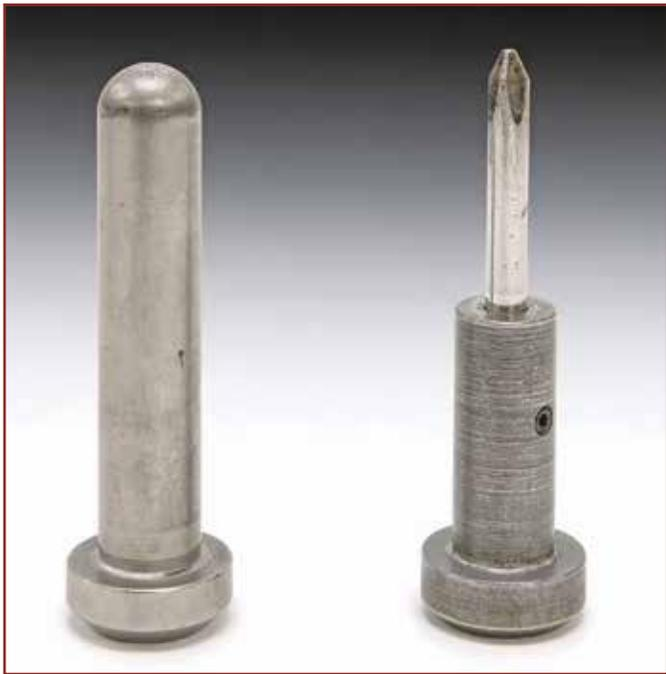
Figure 4 – Left: impactor specified in ASTM D4226; right: modified impactor with Phillips #2 screwdriver tip.
