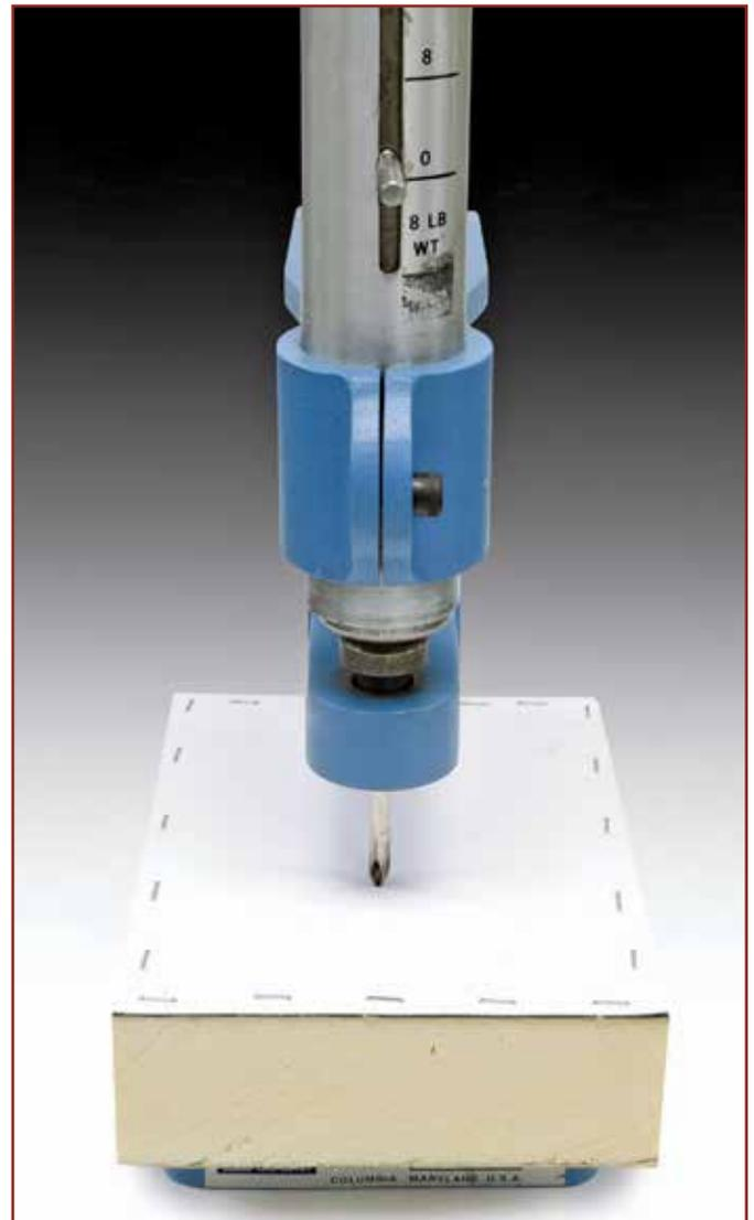
Figure 5 – Impact-resistance setup. Left: setup for unsupported membranes; right: setup for supported membranes.
