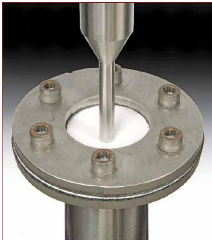
Figure 1 – Clamping of a specimen in the ASTM D4833 Puncture Test. Before and during penetration shown at left and right, respectively.
