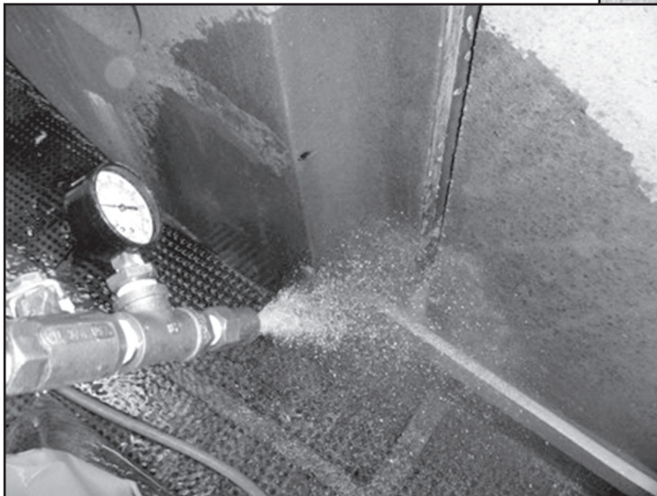
Photo 7 – Leak testing performed via handheld spray nozzle in accordance with modified versions of ASTM test methods.
