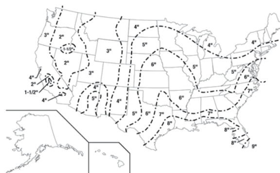
Figure 1 – Storm drainage sizing precipitation rate in inches/hour, based on 15-minute precipitation. Precipitation rate maps help designers create the best drainage systems for an area, given expected rainfall.
