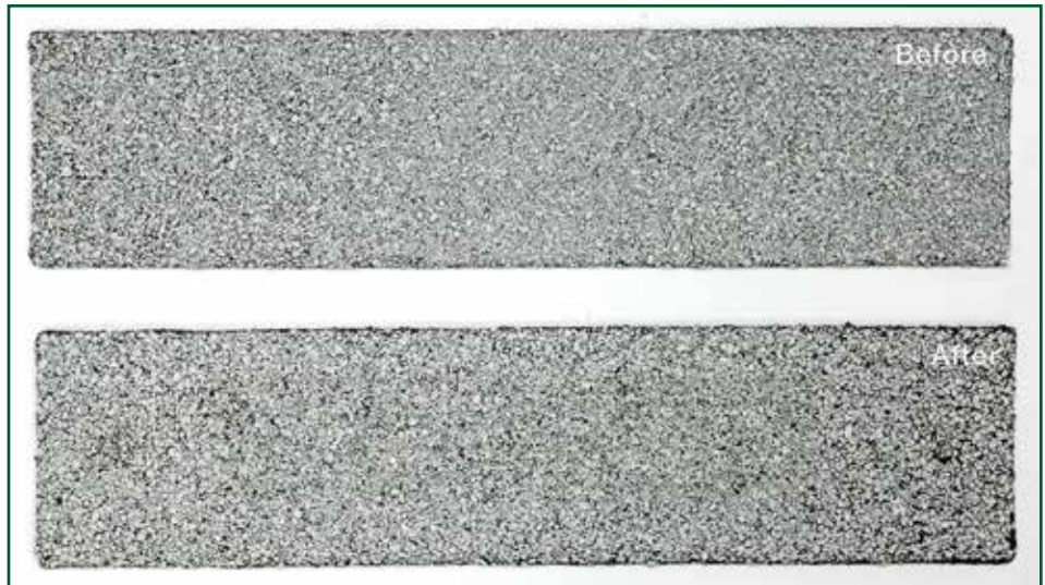
Figure 4 – ASTM D4977 scrub panel of a polyurethane-modified bitumen membrane before and after aging in California for about six months.
