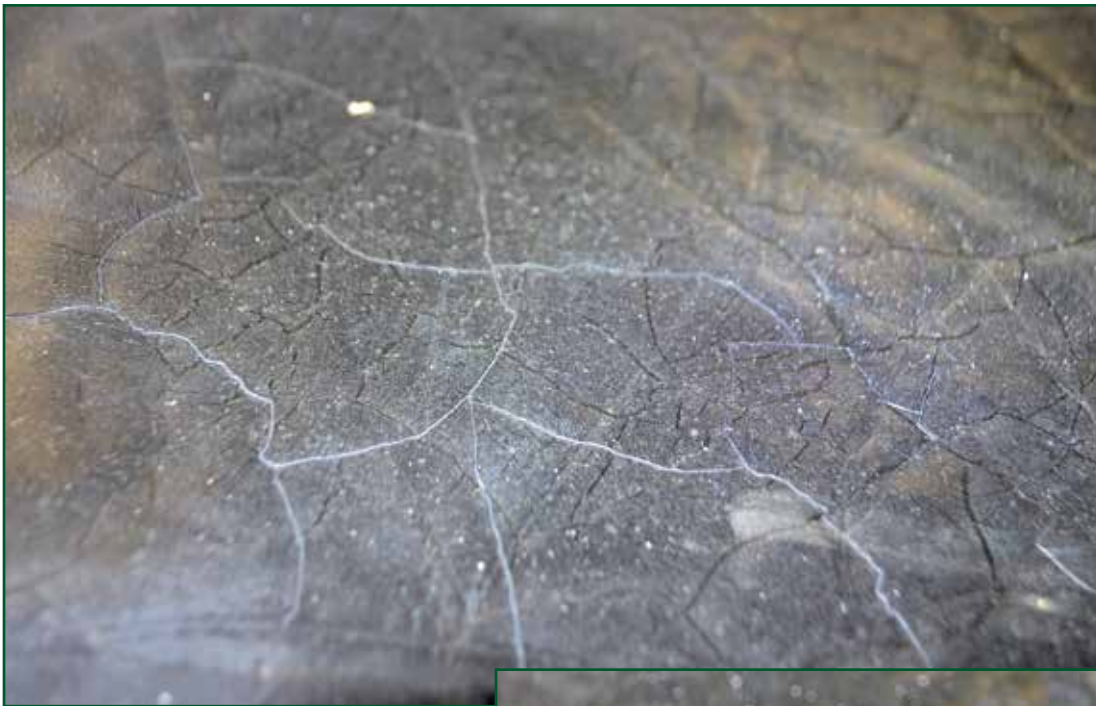
Figure 1 – Surface of polyurethane-modified bitumen that has been exposed to unfiltered ultraviolet radiation for 1,500 hours.
