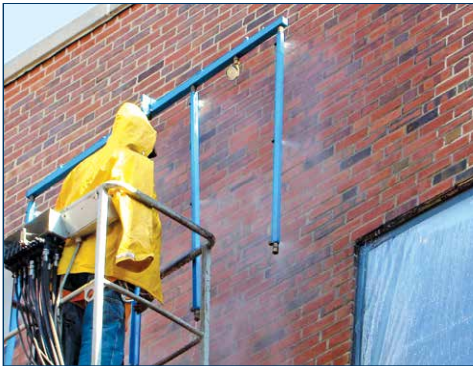
Photo 7 – Calibrated spray rack testing performed on mass masonry wall with adjacent window opening masked to isolate the masonry.
