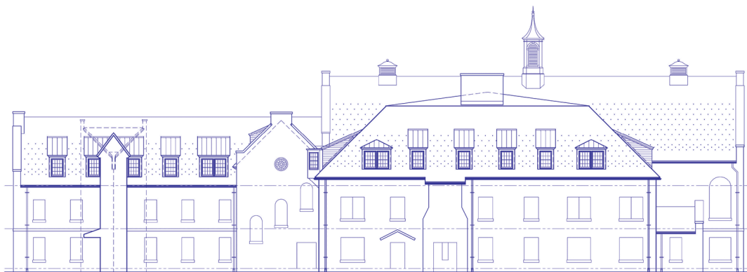
Figures 9A (above) and 9B (right) – Architectural renderings of the existing and proposed dormer reconfiguration.
