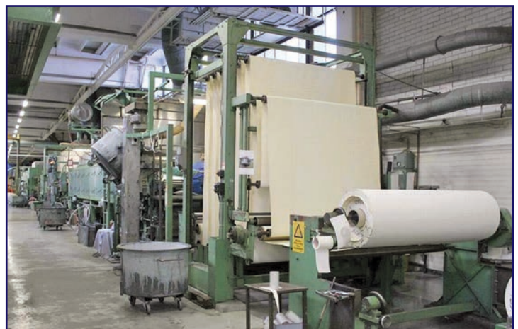
Figure 1 – Knife-over roll coating line.
