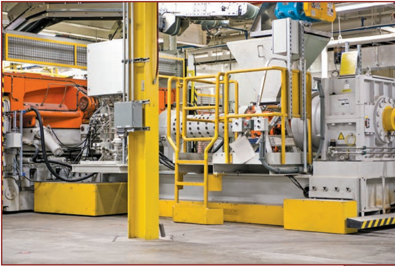
Figure 4 – Extruder in an EPDM roofing plant. Two extruders are utilized—each making a separate sheet that will become one homogenous membrane.
