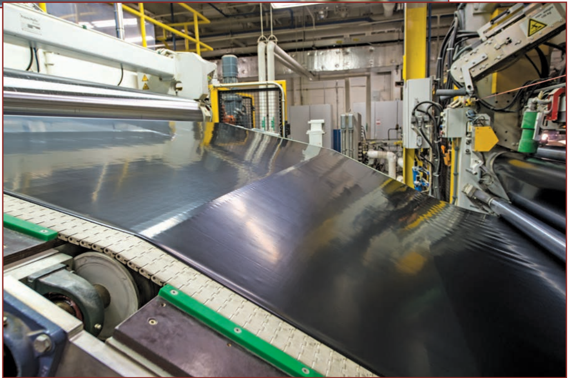
Figure 7 – Extruded membranes have exceptional surface finish and consistency.
