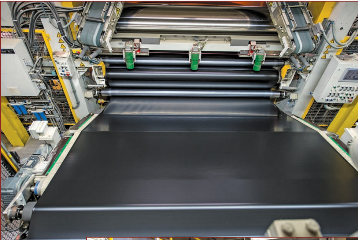
Figure 6 – Extruded membrane prior to entering the doubling roll that will combine two layers into one membrane.
