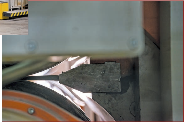
Figure 5 – EPDM material exiting the lip of the die.
