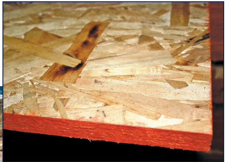
Figure 2 – OSB has strands with specific length-to-width ratios generally lying in the panel's long direction; these are on the order of 1 to 2 in. wide and 6 to 9 in. long, layered and combined with wax and resin adhesive.
