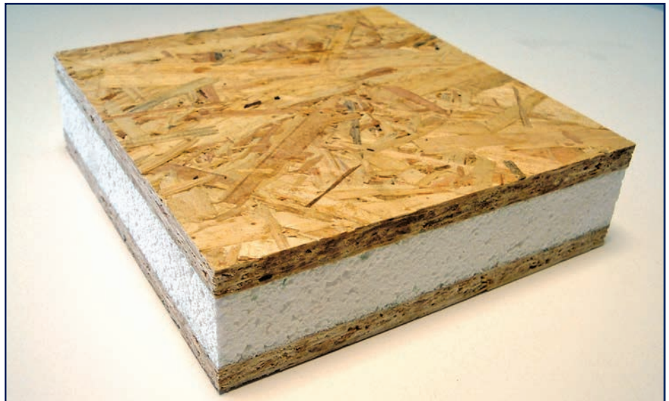
Figure 3 – OSB can be coupled with other materials and marketed as a composite or sandwich product having insulation, such as bead polystyrene; these structural insulated panels are becoming quite popular.
