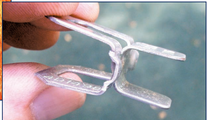
Figure 7 – Clips are not intended to be the spacing element between panels. They do provide that incidental function, but their purpose is to reduce the effective spacing of framing members.
