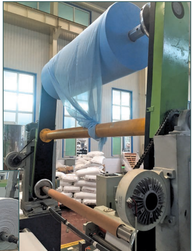
Figure 21 – Nonwoven fabric roll ready for lamination.
