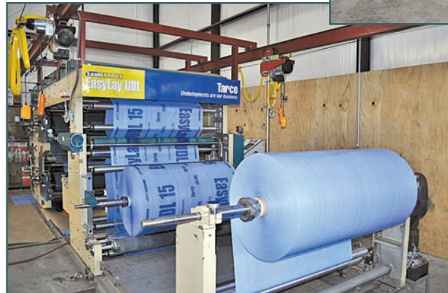
Figure 25 - Winding into small rolls.
