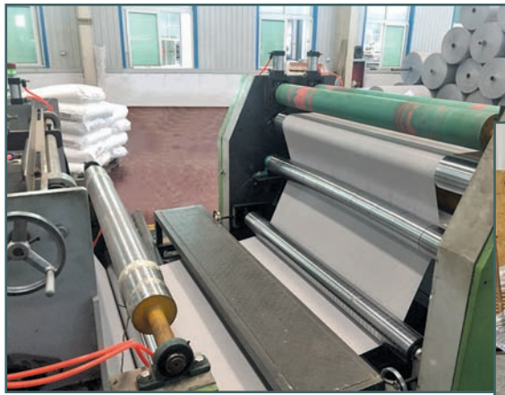
Figure 25 - Winding into small rolls.
