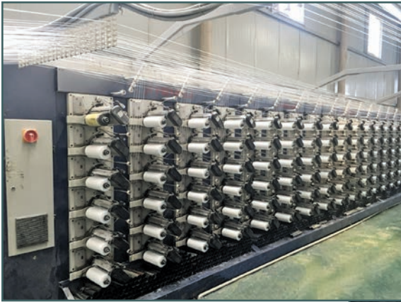
Figure 15 – Winding filaments into spools.
