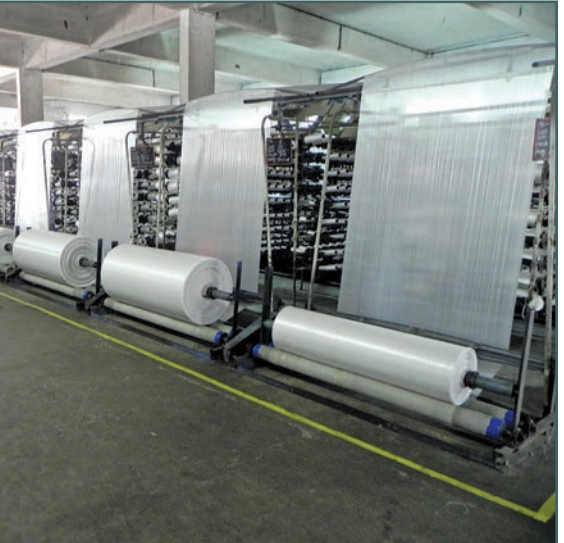
Figure 19 – Winding scrim into rolls.
