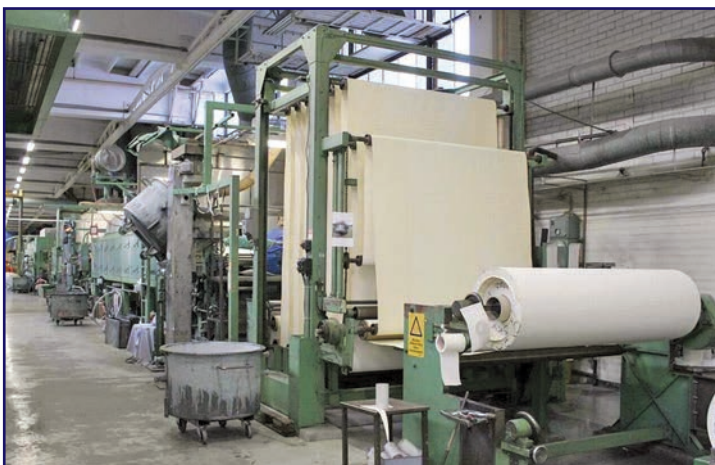
Figure 1 – Knife-over roll coating line.
