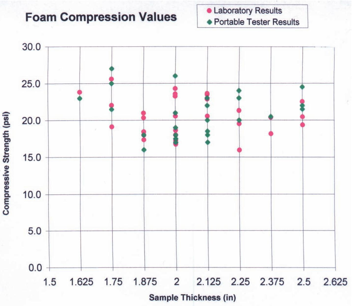
Figure 9: Strength vs. Thickness distribution.
