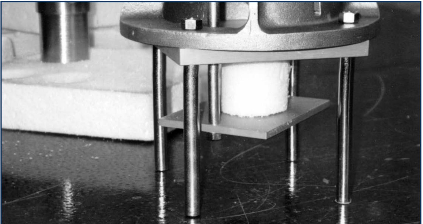
Figure 5: Portable Foam Compression Tester.
