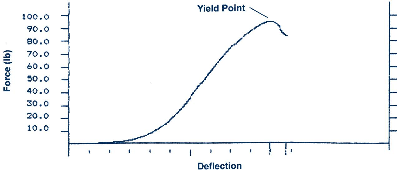
Figure 7: Typical results from laboratory compressive strength test.
