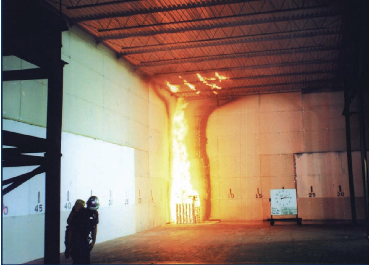
*Above: 25-Foot Corner Test, 14 minutes into the 15-minute test.*
