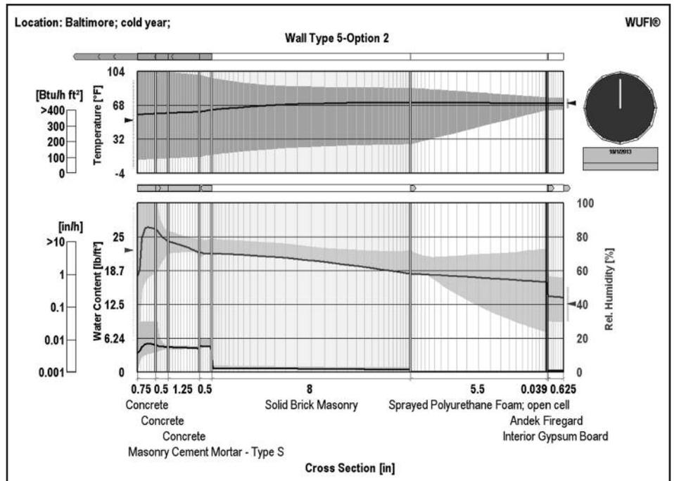
**Figure 8 – View of a graphic output from the hygrothermal analysis of a rehabilitation option of historic masonry-wall system using WUFI. The restoration option (described in Figure 5) allows the brick masonry to dry to the interior and exterior, resulting in acceptable levels of moisture within the brick masonry as indicated in the resulting graph.**
