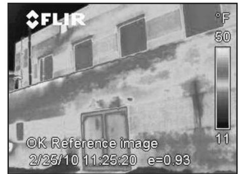
**Figure 3 – View of a thermal image of a masonry building with window openings and a metal door. Note the higher temperatures are darker (reds and yellows in full color), indicating heat loss through the window glazing and frame metal door as well as the lower parapet in the photo.**
