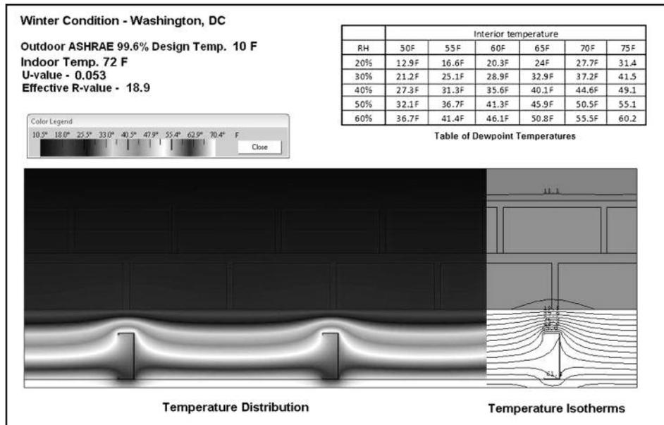
**Figure 5 – View of a graphic output from a thermal analysis of a rehabilitation option for a masonry wall system using THERM. The original wall included precast panels set into the face of solid brick-masonry backup. The rehabilitation option shown includes adding open-cell (½ lb/cu ft) spray-foam insulation inboard of the brick masonry and between steel studs that support interior finishes.**
