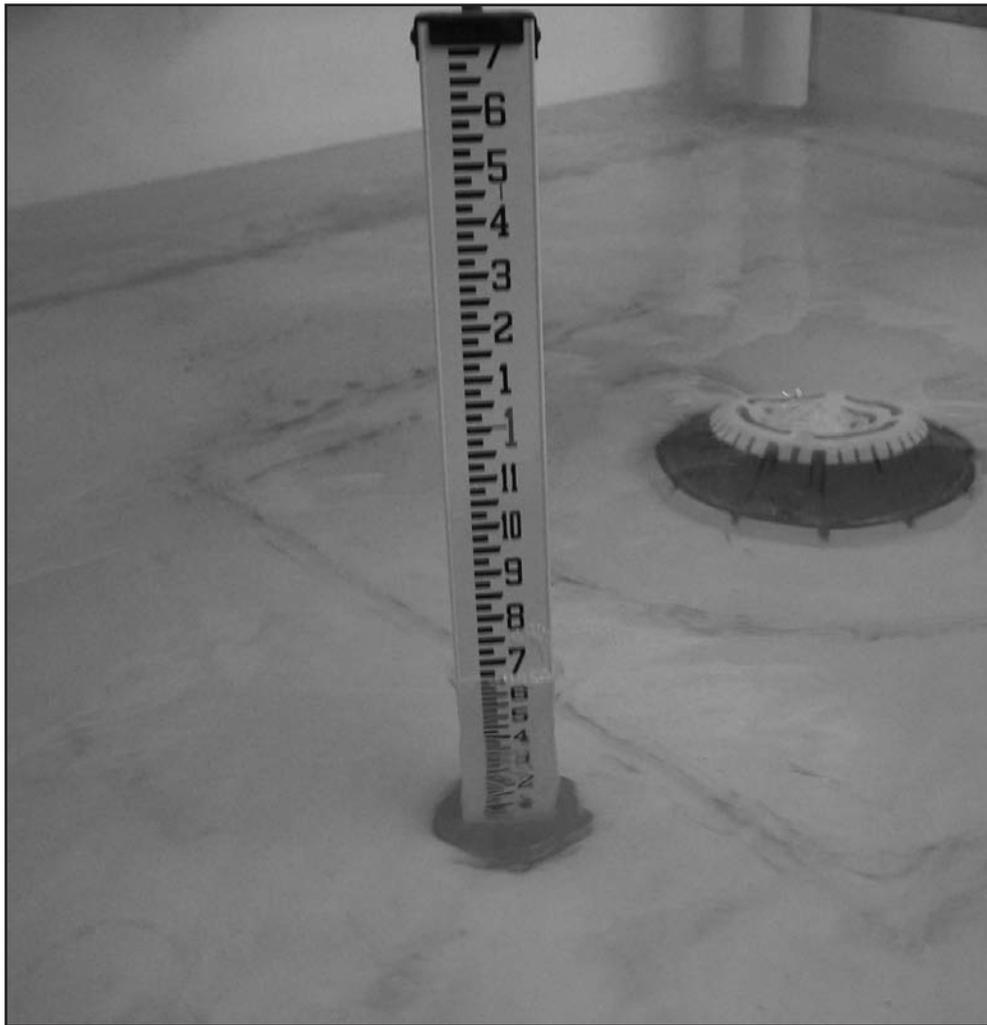
ected to pumps and a water reservoir. Different types of drain devices were flooded at incremental flow rates of 200, 400, 600, and 800 gallons per minute. As water was pumped at different flow rates, the depth of water accumulation was measured.
