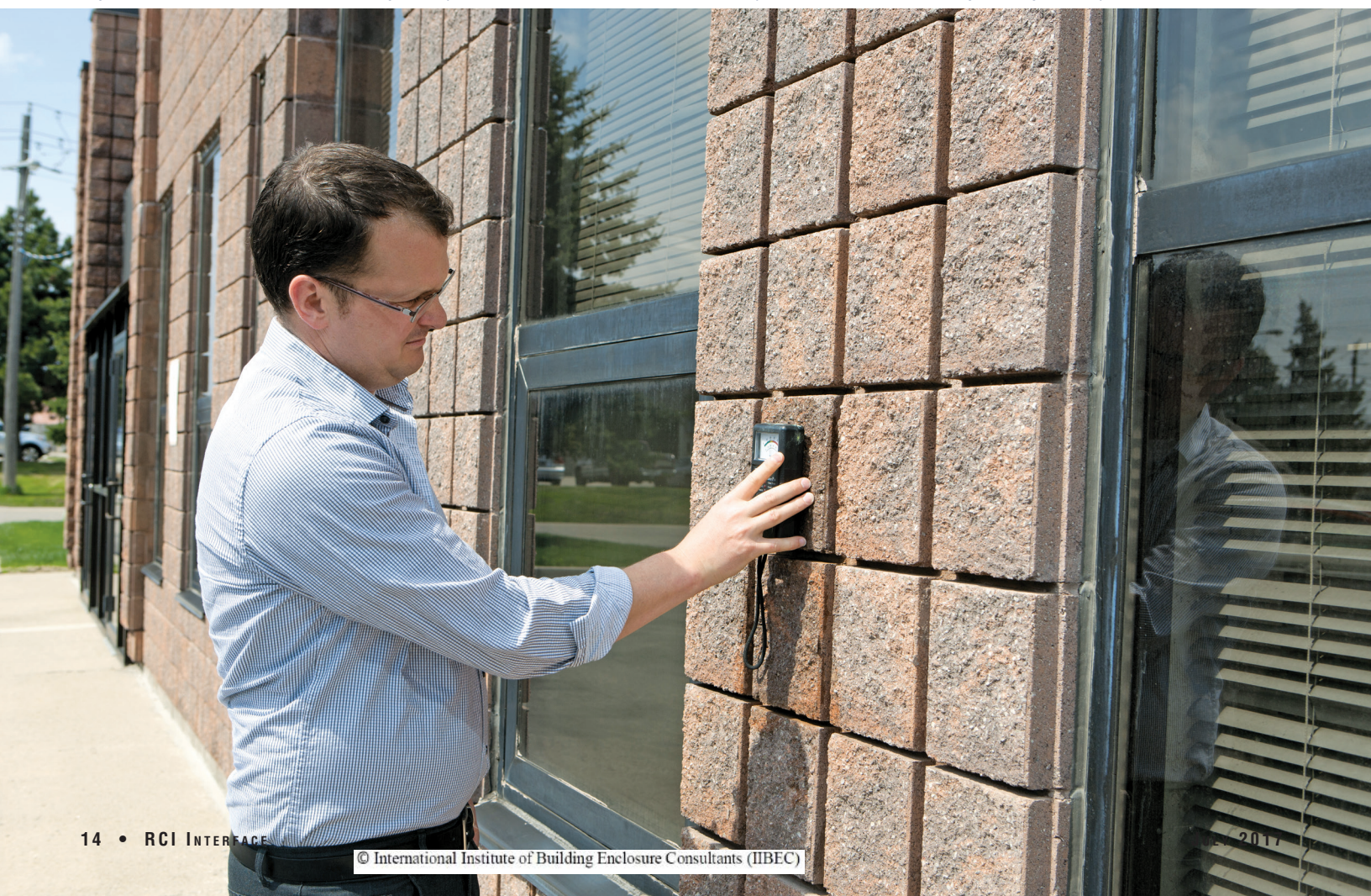
Figure 5 – The author demonstrating use of a moisture content meter as part of nondestructive masonry testing in the field.
