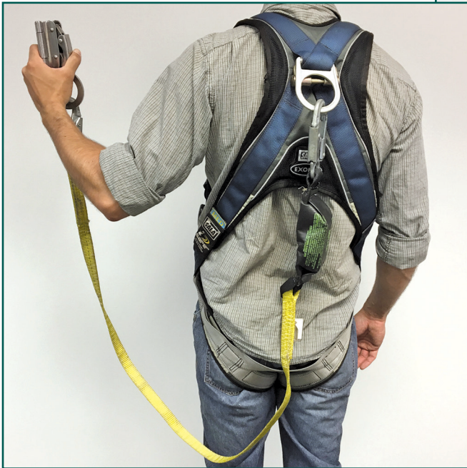
Figures 1A and 1B – Two types of lanyards are pictured. 1A (below) incorporates a shock absorber for fall arrest, and 1B (right) is for fall restraint.
