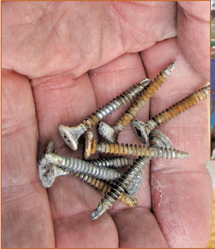
Photo 3 – Self-drilling tapping screws are equipped with hardened tips that resemble a drill bit. These 1¼-in. bugle-head fasteners had “the ability to drill their own hole” through the stainless steel components shown in Photo 2.
