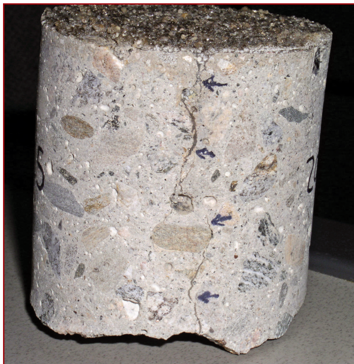
Figure 5 – Test core showing epoxy penetration to the bottom of a crack.
