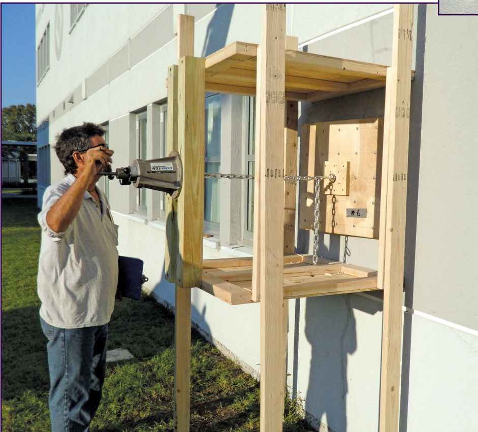
Figure 3 – Example of test frame and pull testing setup.
