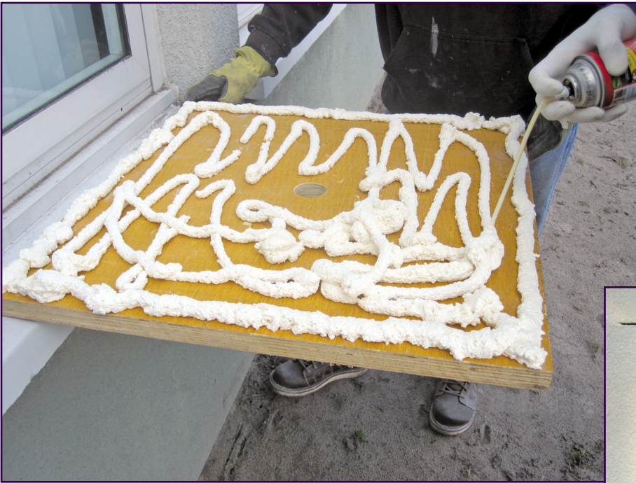
Figure 1 – Example of disposable wood bonding panel to be adhered to stucco test specimen. Note photograph is for demonstrative purposes only, as expandable foam adhesive is prohibited per ASTM C1860.
