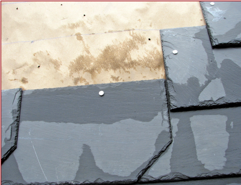
Figure 5 – Wetting of rosin paper and within top lap when water was sprayed at an upward angle.
