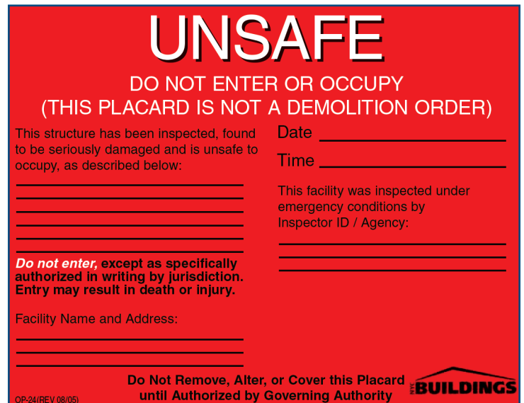
Figure 2 – Red-colored “Unsafe” tag used during rapid evaluation. 7
