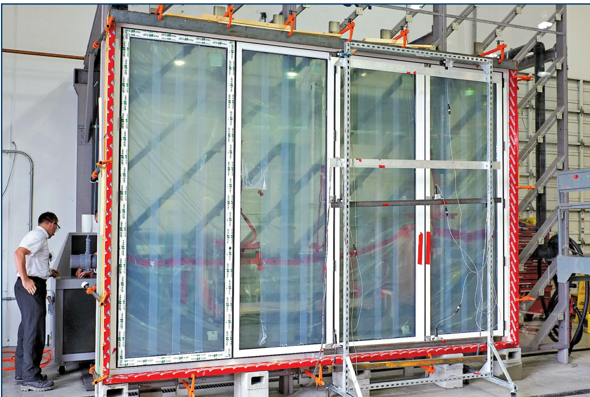
Figure 1 – Folding door undergoing lab structural testing to the NAFS standard. Photo by Al Jaugelis.
