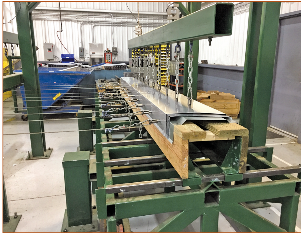
Figure 5 – In the RE-3 test, simultaneous simulated wind loads are applied on both vertical and horizontal surfaces.
