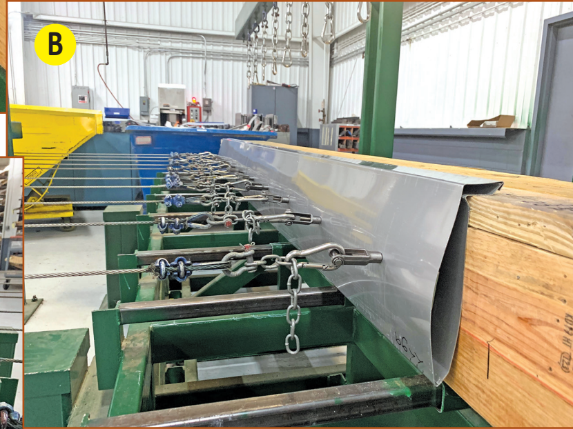
Figures 4A, 4B, and 4C – In the RE-2 test, a distributed load is applied to the vertical face of the fascia in order to simulate the pressure created by wind velocity.
