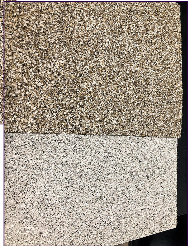
Figure 11 – Close-up comparison of stained granules vs. non-stained.
