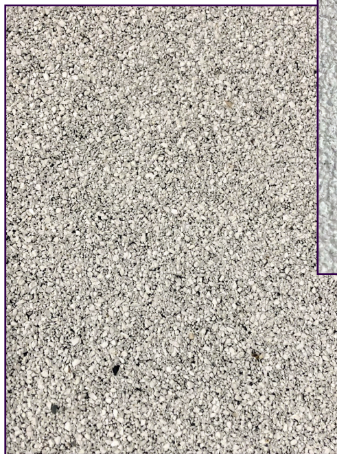
Figure 1 – Close-up of granules on “cool” cap sheet with white-colored granules.
