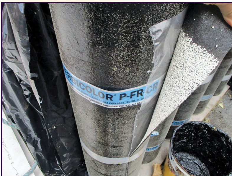
Figure 15 – Film on roll to prevent staining of granules.
