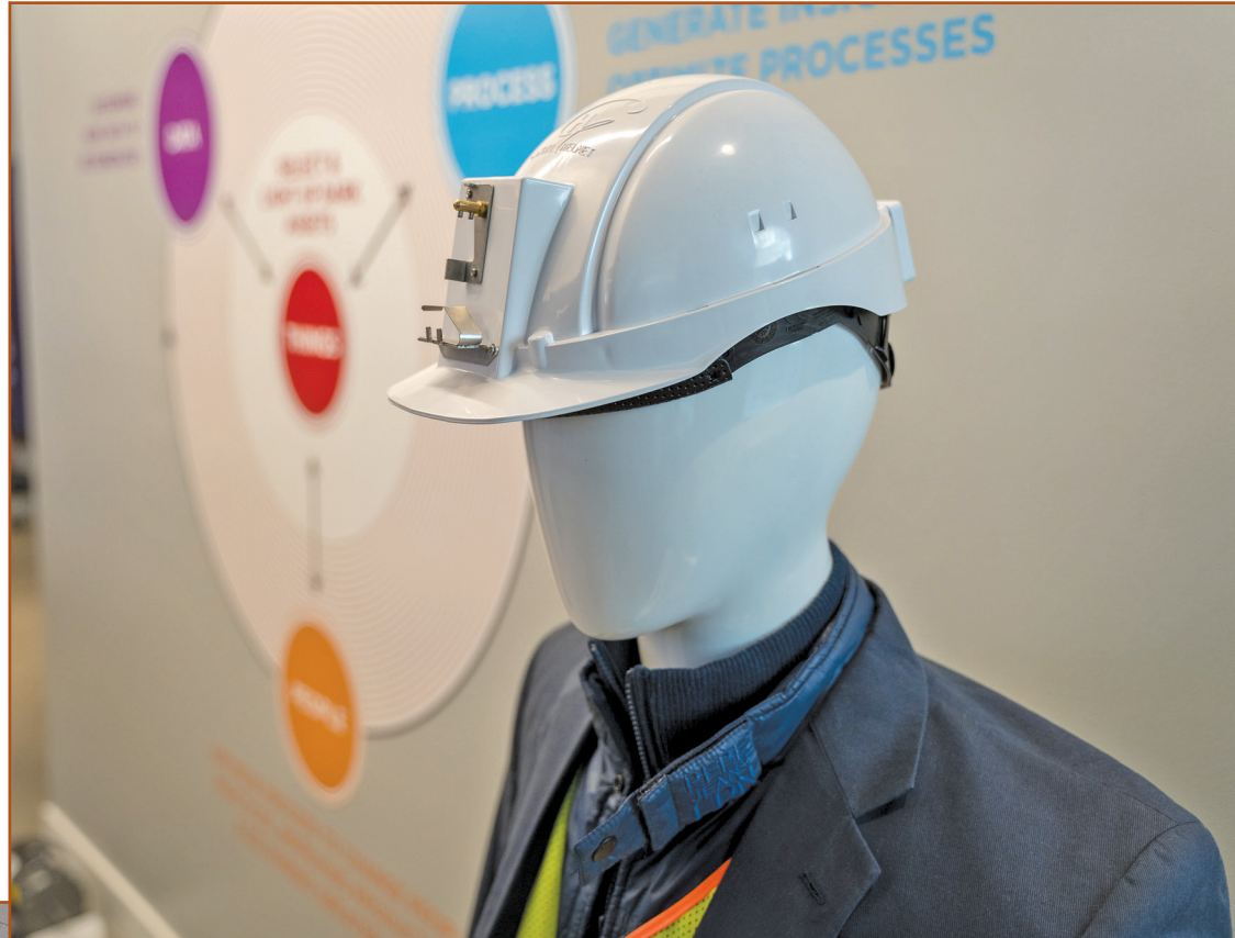
Figure 2 – A hard hat equipped with technology to monitor impacts and worker vital signs was one of the items being developed in the Microsoft Innovation Lab.
