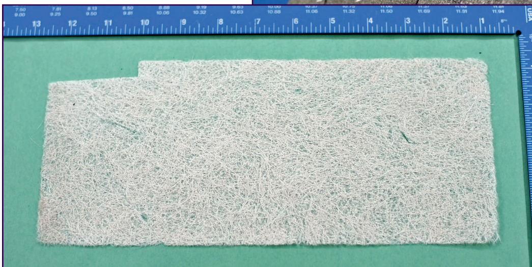
Figure 2 – Roofing membrane after being desaturated in vapor degreaser.
