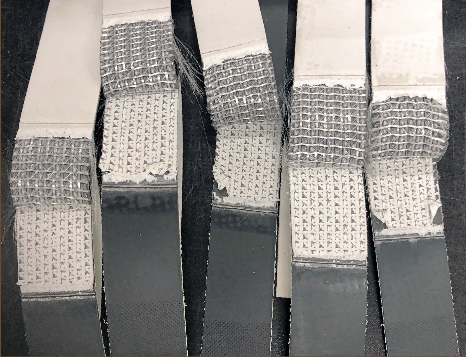
Figure 12 – Film tearing bond of nearly 100 percent, from Location 6.
