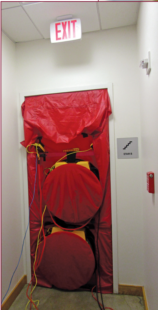
Figure 3 – Setup of blower door for airtightness testing.
