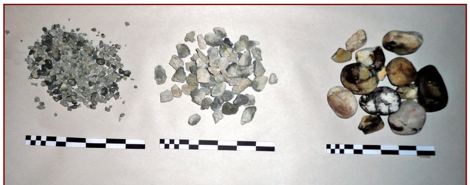
Figure 2 – Samples of aggregate from evaluated roof systems after hurricane events (Morrison, 2011). Photo courtesy of Deer Ridge Consulting Inc.
