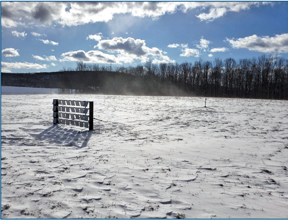
Figure 8 – Installed in a large open field in a high-wind area of rural western Pennsylvania, the wind-driven kinetic façade test unit was exposed to varying wind conditions, and the wind-induced sound was measured and correlated with the wind parameters.
