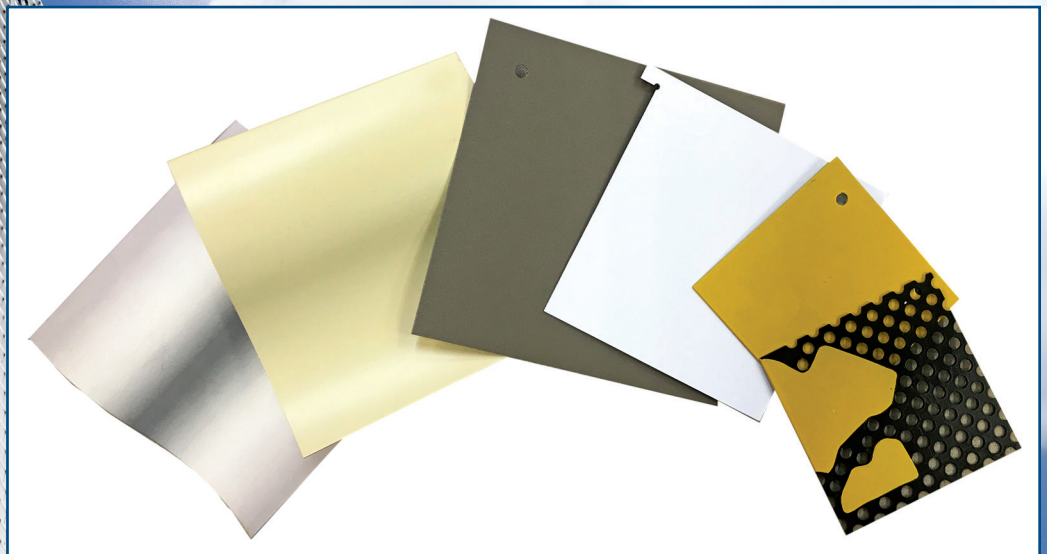
Figure 2 - While aluminum is the most popular material for flappers in wind-driven kinetic façade systems, other options include perforated materials, stainless steel, polycarbonate, PTFE, acrylic, and even PVDF films.
