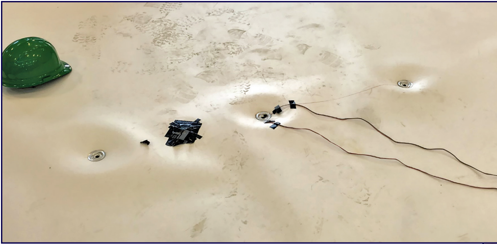
Figure 6 – A photograph showing circular permanent upward membrane deformation due to two-directional loading in Test 2.
