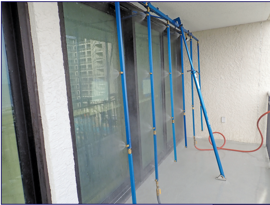
Figure 2. View of water penetration testing.
