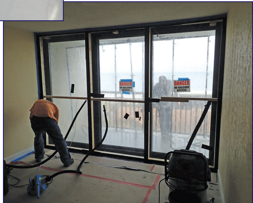
Figure 2. View of water penetration testing.
