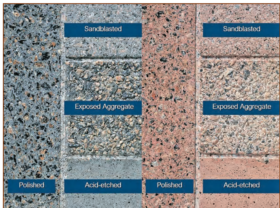
Figure 1. A variety of precast concrete finish options within two different concrete mixture designs.
