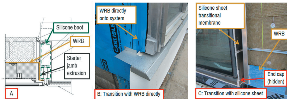
Figure 10. Transition options to curtainwall jamb: (A) detail; (B) transition with WRB directly; and (C) transition with silicone sheet. Note: WRB = weather-resistive barrier.
