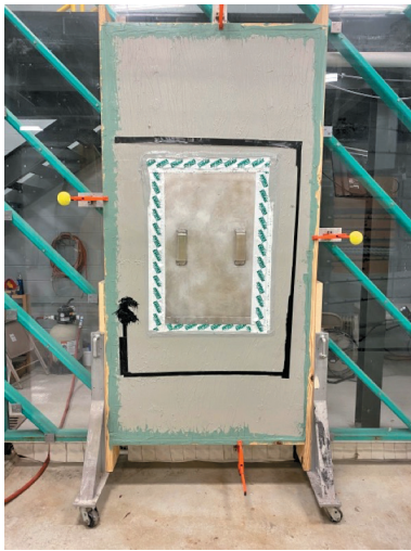
Figure 3. Mock-up 1, round 2 testing, fluid-applied water-resistive barrier system.
