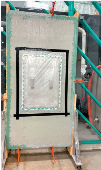
Figure 10. Mock-up 3, round 2 testing during blank isolation air-leakage testing.
