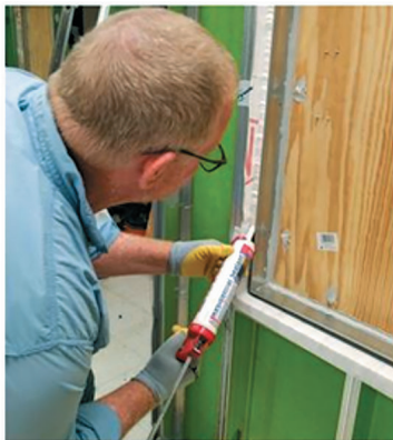
Figure 7. Mock-up 5, round 1 testing, mechanically fastened WRB system. Note: WRB = water-resistive barrier.
