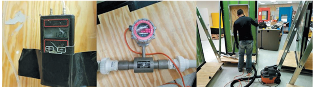
Figure 11. Air-leakage testing equipment (manometer, airflow meter, commercial vacuum).
