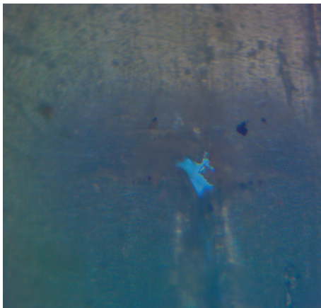
Figure 7. A 100× image of a micropore in a woven building wrap.
