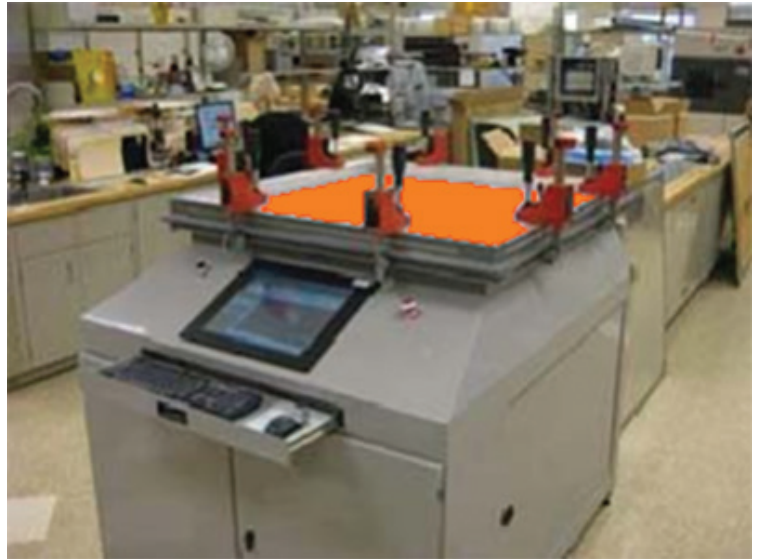
Figure 17. Equipment used to test air permeance using the ASTM E2178 test method. 15
