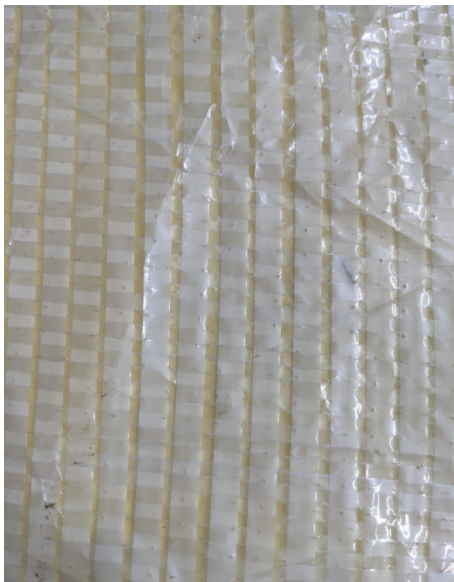
Figure 3. A woven, microporous building wrap provides vapor permeability.
