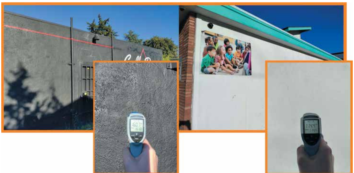
Figure 2. The temperature difference between a dark and light wall taken on July 19, 2022, at 7 p.m. in Portland, Oregon.
