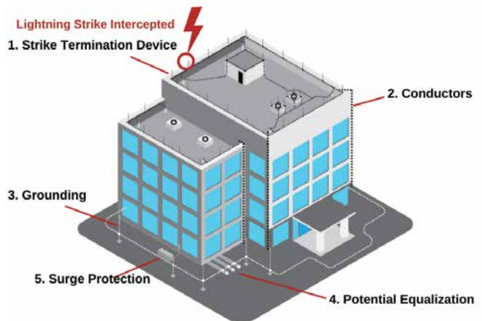
Figure 3. This model shows the basic design of a lightning protection system; lightning is intercepted by a strike termination device.
