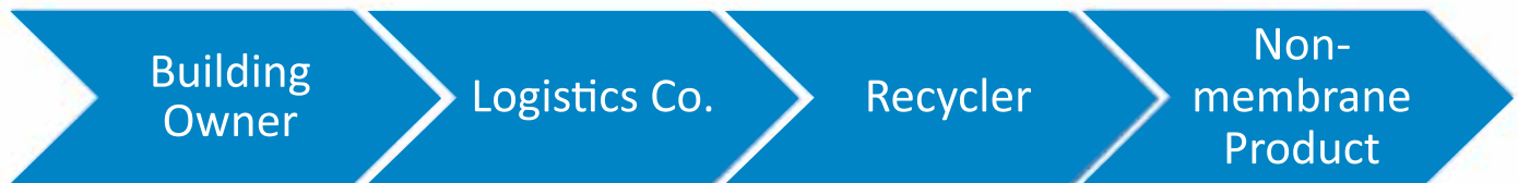
Figure 5. Open-loop recycling. The PVC membrane manufacturer specifies recycling with the owner. The recycler then sells to the open market.
