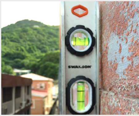
FIGURE 6. A level/straight edge was used to show the precast concrete substrate behind the stucco was out of plane.
