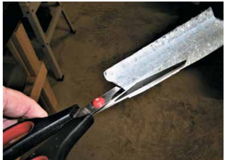
Figure 11. This light-gauge metal liner can be cut with household scissors. There is no wind rating whatsoever to be had when materials are fastening with screws to this type of liner.
