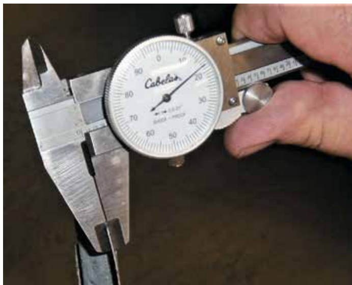
Figure 10. Micrometer measurement confirms that this 26-gauge (0.017-in.) metal liner is not intended to hold fasteners.
