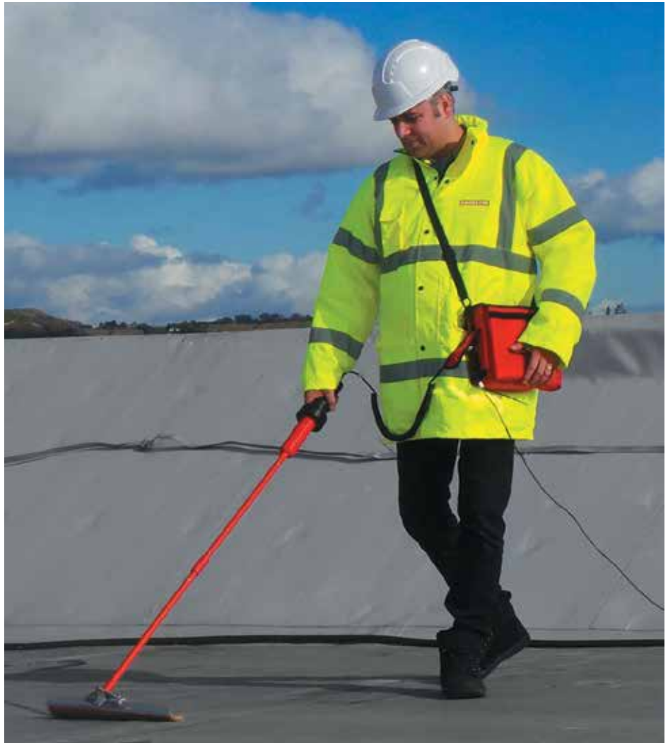
Figure 4. High-voltage spark/holiday testing.
