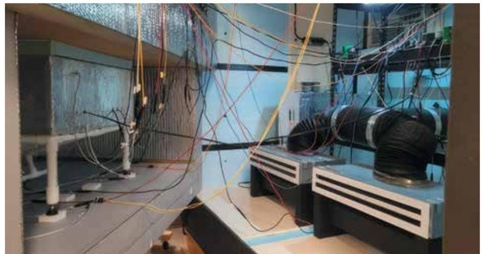
**Figure 3.** Open view of assembly frame and meter boxes (left) and guard box with climate control (right) within the climate chamber.
