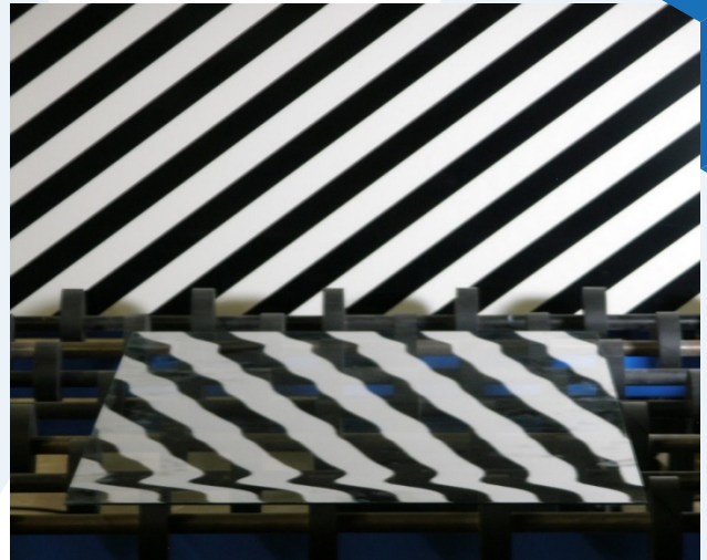
FIGURE 1. Zebra board visual evaluation of glass distortion on heat-treated glass.
