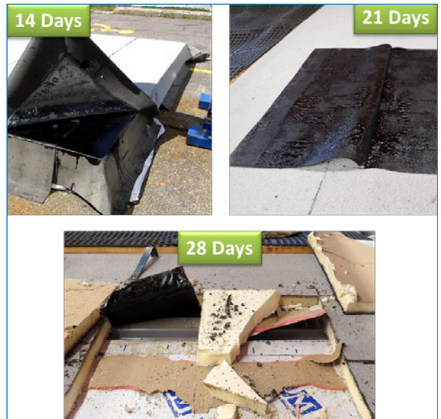
FIGURE 22. Failure modes varied with curing time for an AARS.
