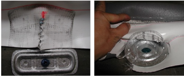
FIGURE 20. Fastener plate/membrane engagement against wind uplift in MARS.
