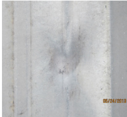
FIGURE 12. Photograph of a cleaned hail-caused dent—note the absence of evident corrosion.
