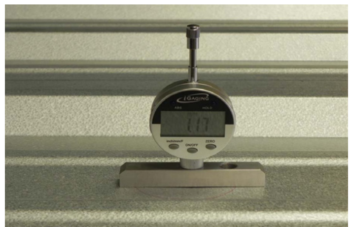
FIGURE 3. A field dent depth measurement.
