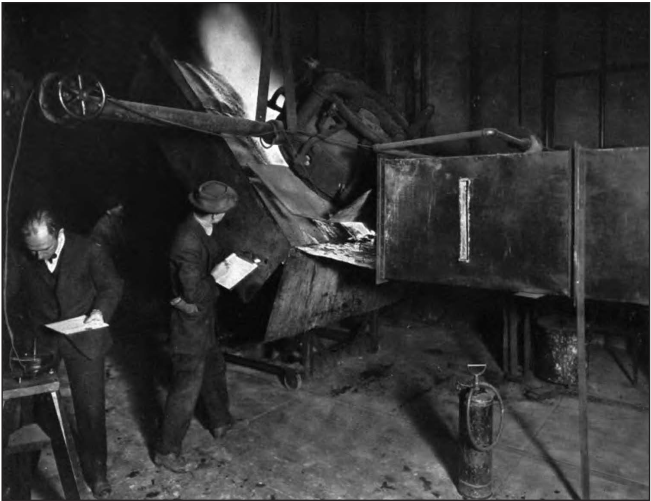
Figure 1 – One of the earliest test apparatus used by the Underwriters Laboratory for testing of roof coverings.
