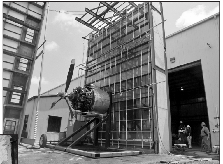
Figure 5 – Airplane engine used during dynamic water penetration testing of laboratory mock-up.
