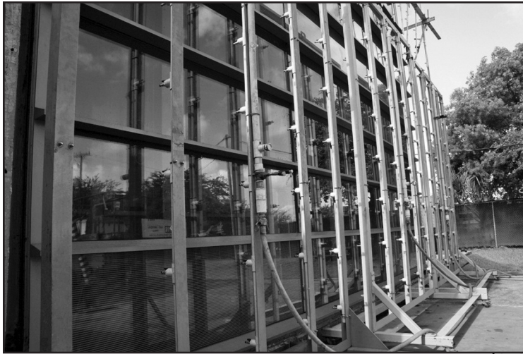
Figure 3 – Spray rack installed in front of large curtain wall system during laboratory mock-up testing.
