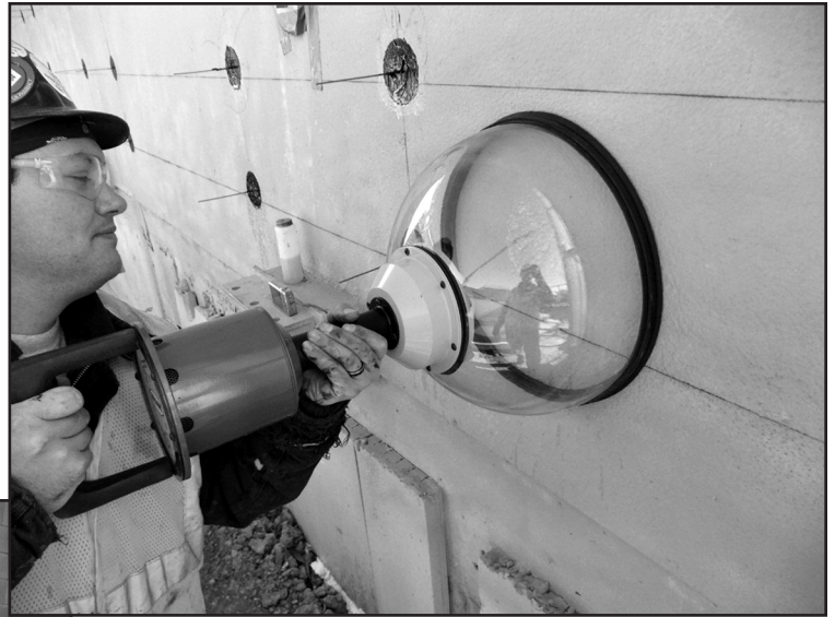
Figure 10 – Air leakage testing of insulation fastener. ASTM E1186.
