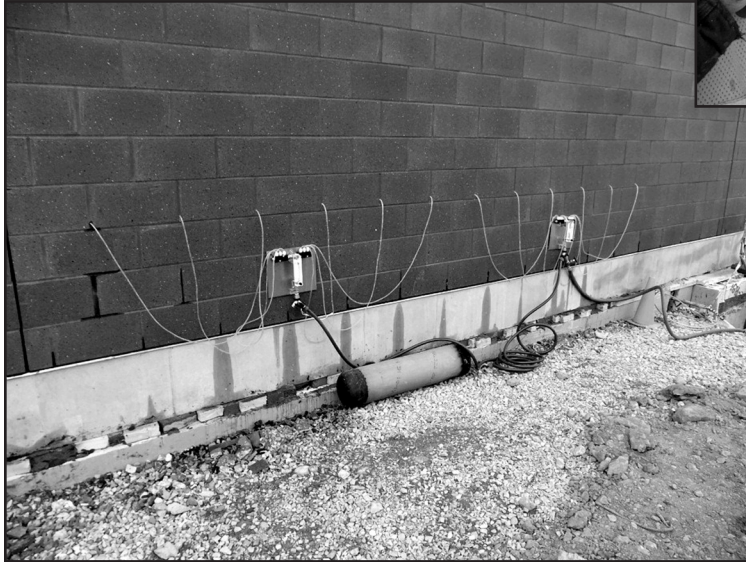
Figure 9 – Cavity wall drainage testing on newly constructed cavity wall. ASTM C1715.
