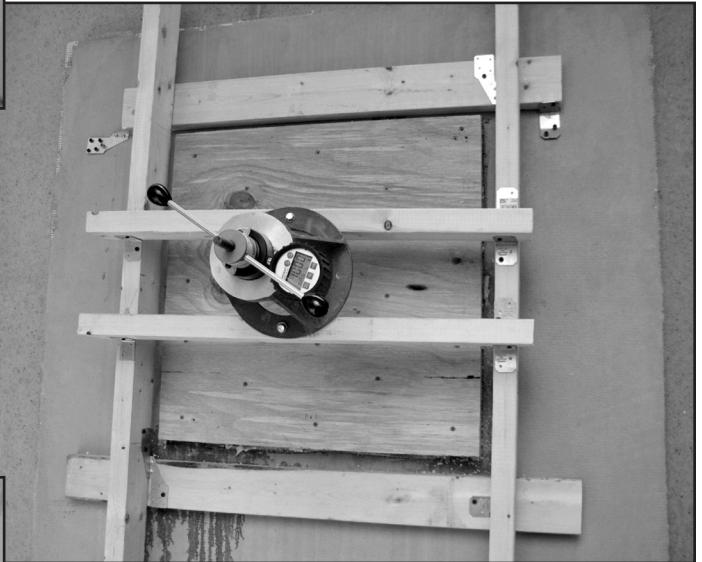
Figure 13 – Pull testing of EIFS mock-up. ASTM D4541.
