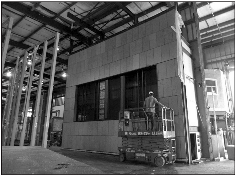
Figure 1 – Example of a simplified lab mock-up containing a punched window opening and rainscreen stone panels.
