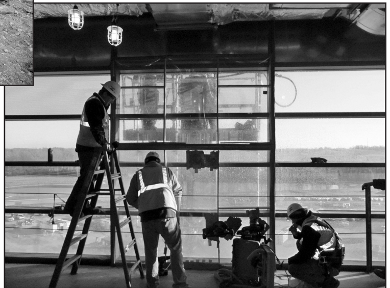
Figure 11 – Air leakage and water penetration testing of newly installed curtain wall unit. ASTM E1105 and ASTM E783.
