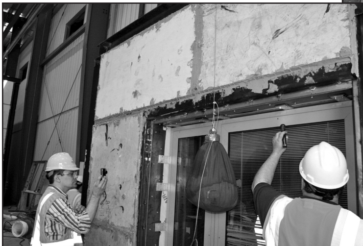
Figure 6 – Laboratory setup for impact testing of a window assembly.
