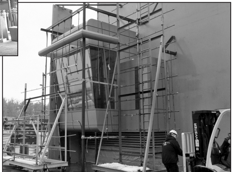
Figure 2 – Example of complex lab mock-up containing curtain wall, louvers, metal panels, and multiple inside- and outside-corner conditions.
