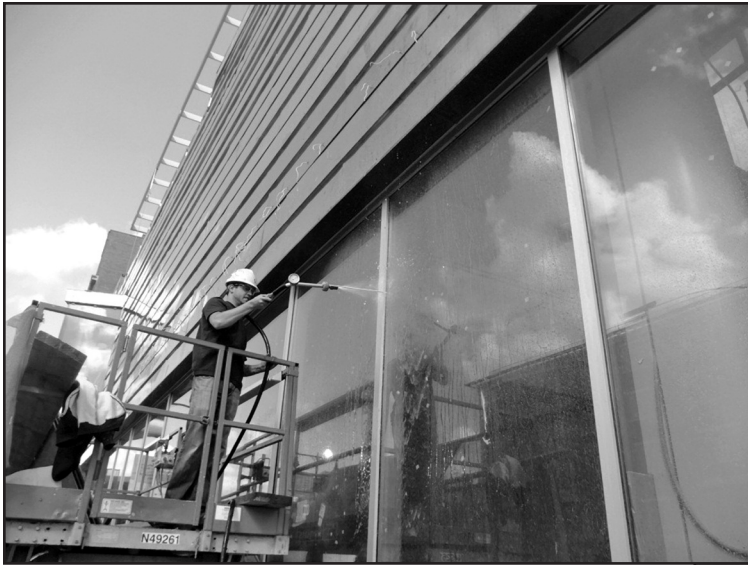
Figure 12 – Water penetration testing of curtain wall system. AAMA 501.2.
