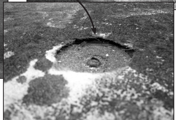
Figures 6A, 6B, and 6C - Failure mode of System 1. The add-on remains on top of the membrane after the dynamic wind test. Only fasteners and metal plates pulled through the support board.
