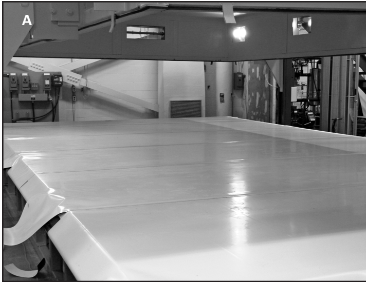
Figure 9A - 9H - PV module response for Systems 1 and 2 during dynamic wind testing.
