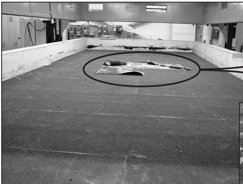
Figures 6A, 6B, and 6C - Failure mode of System 1. The add-on remains on top of the membrane after the dynamic wind test. Only fasteners and metal plates pulled through the support board.
