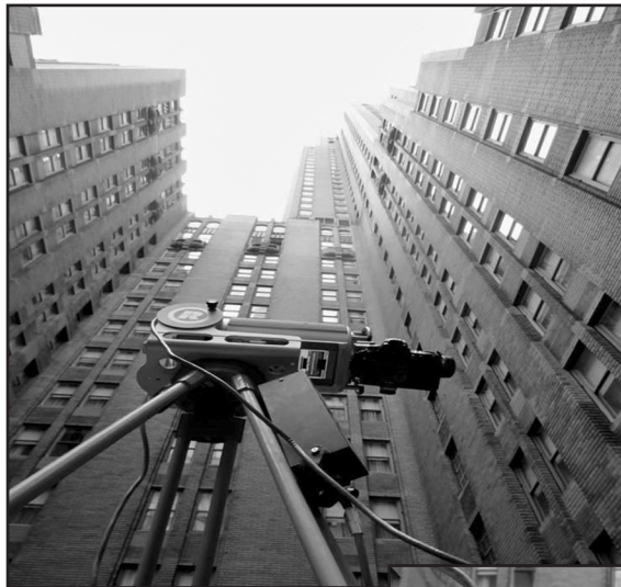
Photo 3 - Typical scanner set up on tripod.
